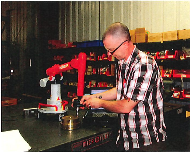
PRECISE WORK: Jason Dodge, a Grade 1 inspector in Micro Precision's Quality Control Department, works on a Romer Arm. Photo by Jan Tormay
